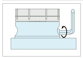
2.1 Loosen the clamping bases cam cylinder fully. Measure dimension of the jaw for machining. Tighten the cam cylinder until each jaw section expands a further 0.15mm beyond desired clamping dimensions.
