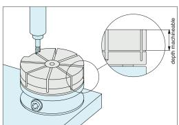
2.2 Machine the jaw to the contours of workpiece. (Do not machine the jaws beyond the machinable depth – see data tables of jaws 12056 and 12057 for dimension.
