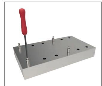
Install the Xpansion pin's tapered drive screw into fixture plate.
