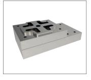
Run first operation – note the clear tooling path possible with no noticeable external clamping interference.
