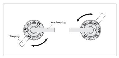
Two clamping and unclamping positions of handle can be chosen for 12085.W0008/W0108
