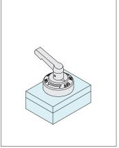
2. Insert the clamper to the bushing.
