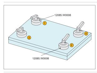
Ensure the handle os positioned at 'OFF' marke and lift down the fixture plate.
