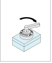
3. Turn the handle to 'ON' mark for clamping.
