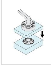
1. Ensure the handle is positioned at 'OFF' mark.
