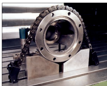
Clamping with the chain clamp set.
