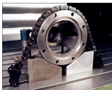
Clamping with the chain clamp set.
