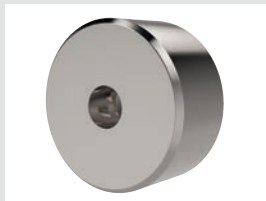
Stainless Steel Pad from 17-4 stainless steel, hardened to Rc 43/46. Mount via tapped or counter bored hole.
