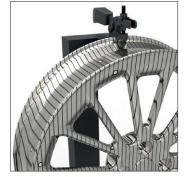
Marking and measuring For overlaying of several pictures, circular markings are attached to the object. A stripe pattern is projected onto the object surface by a white-light projector and photographed by two cameras from different angles of view.
