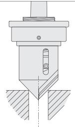
1 When the chamfer tools spindle is lowered, it's pilot cone firstly centres the workpiece before retracting to allow the blade to come into contact with the material and start cutting of the chamfer.
