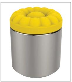
Unique urethane coat prevents marking of delicate components during machining or manipulation by robots. The urethane pad is permanently bonded to the stainless steel body of the gripping pad. With a bubbled texture, air is able to escape and hence avoid any suction action - enabling easy releasing of parts.
